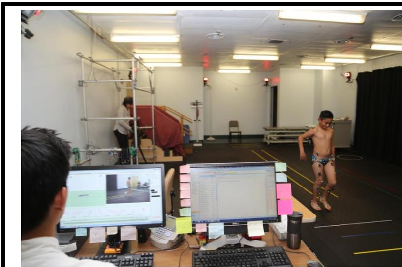
Figure 1. Modern motion analysis laboratory. Patients walk over force plates built into the ground while wearing reflective markers placed at discreet locations, which are recognized by the infrared cameras (8 total), which allows for objective evaluation of joint kinematics and kinetics. Mobile surface-EMG markers have been placed on this patient, which record muscle activity during the gait cycle.
